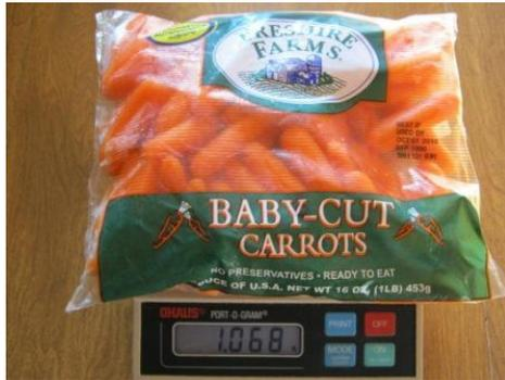
Here's example #1 of W&M Commodity Package Checking -or- Net Weight Compliance. Consumers are only required to pay for the product itself which does not include the packaging (tare weight). The bag of carrots has a posted net weight of 16oz (1 lb), and the scale reads 1.068lb. As a non-destructive test method W&M would determine that this package is in compliance. Every supermarket is required to have a customer scale. Use this scale to compare packages or if you feel a package is underweight.
