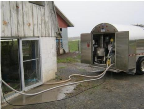
Milk tank testing is conducted on new tank installations or tanks that are no longer in the acceptable tolerance. Milk tank capacities range from 400 to 8000 gallons depending on the size of the farm. The smaller milk tanks can be tested with water using a 5 or 10
