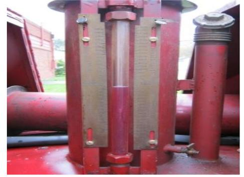
Volume delivery is checked and if necessary, the meter is adjusted, and the test is repeated. Products delivered through vehicle tank meters that have a higher density (such as passenger car and truck motor oils, hydraulic oils, and transmission fluid) are tested gravimetrically (by weight).
