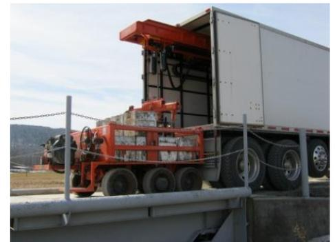
these scales. The W&M department will work with a local scale company for these types of tests. The scale company must provide a certified weight cart and certified weights to conduct these tests. The cart and weights together will weigh in at 25,000 pounds. We then can use substitution weights, such as the weight truck, in order to "build up" to the final test weight of the scale at over 100,000 pounds.
