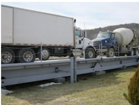
Large capacity vehicle scales are routinely found at salvage yards and gravel pits. Most county W&M departments do not have the required equipment for testing these large scales with capacities of 120,000 pounds and higher. Trucks weighing over 80,000 pounds are routinely weighed on
